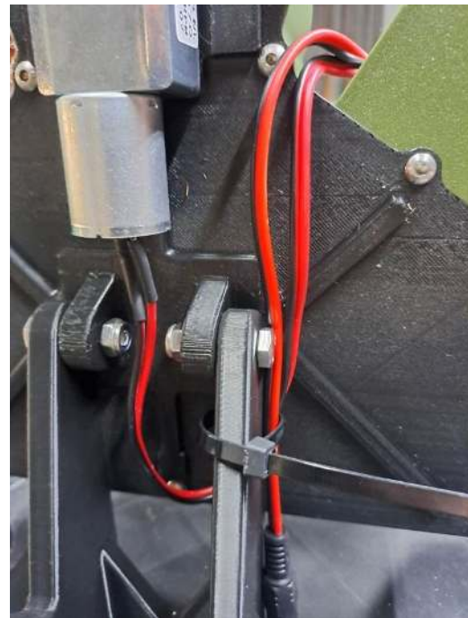
Cable tie position with wiring slack.
