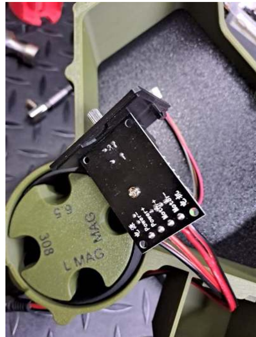
Board markings showing Power and Motor polarity.
