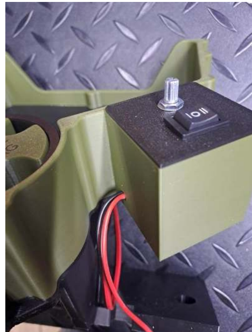
Control panel correctly seated.
