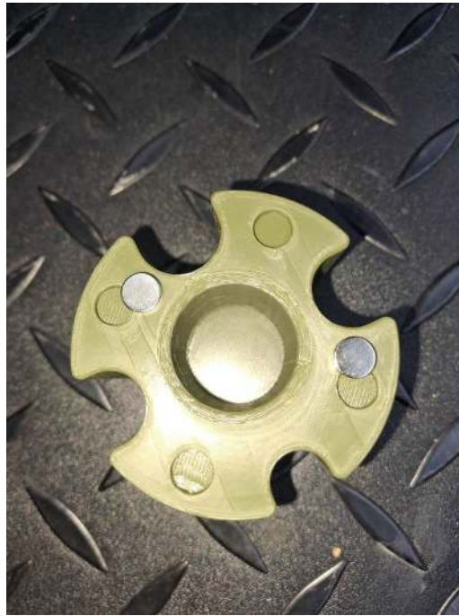
Feed wheel showing installed magnets.
