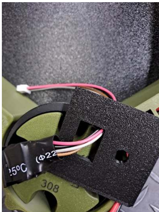
Switch wiring routed through the control cover.
