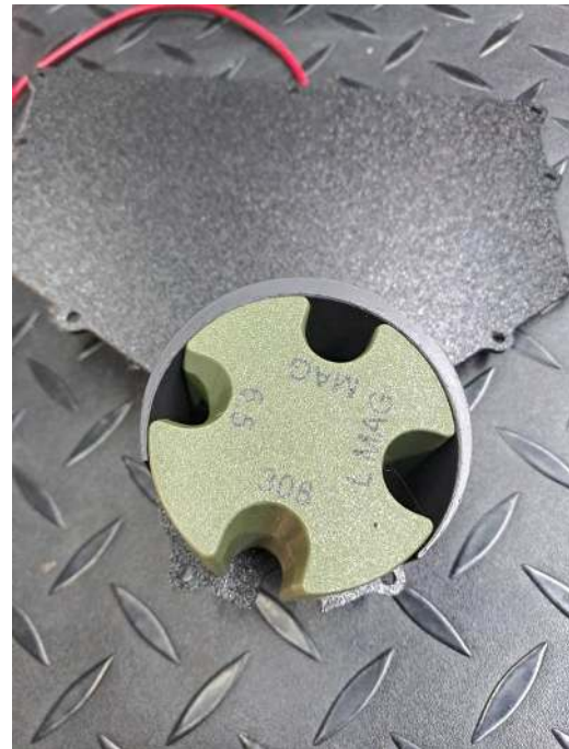
Feed wheel correctly installed.
