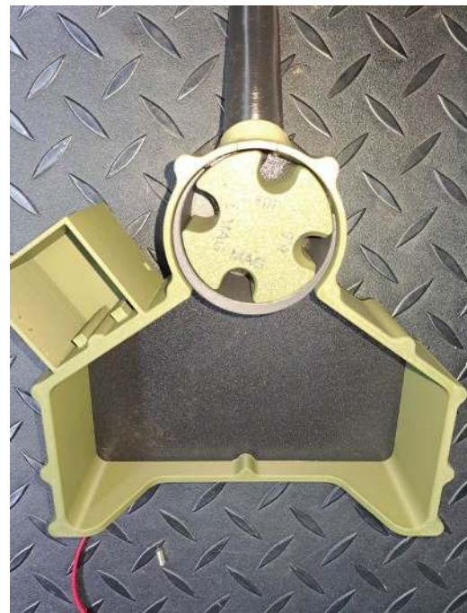
Correct appearance after installation.
