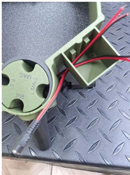
Motor and power wires routed through the same side opening.
