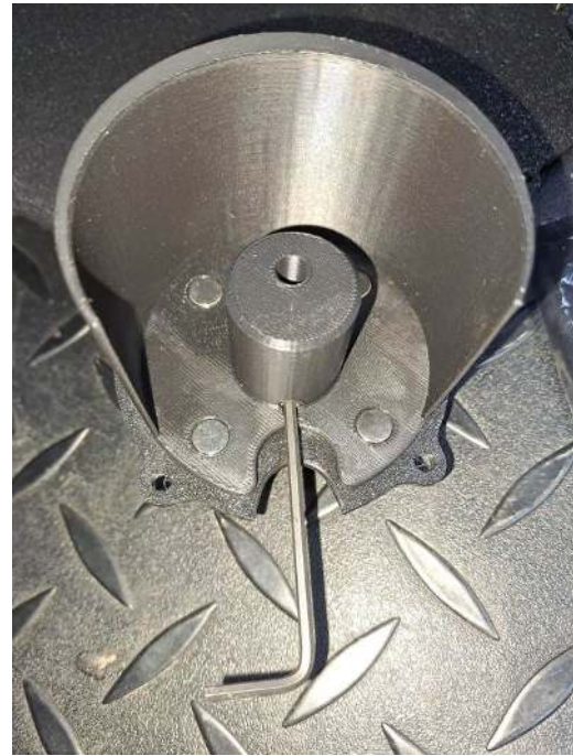
Wheel holder with magnets installed.
