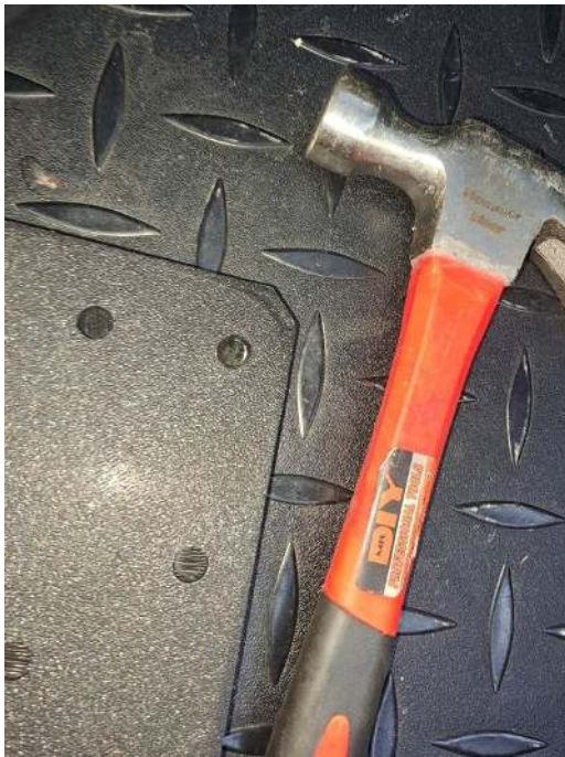
Support the base at the bench edge while tapping magnets in.
