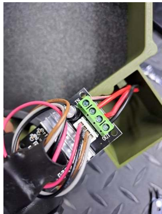
Switch connector plugged into the controller board.
