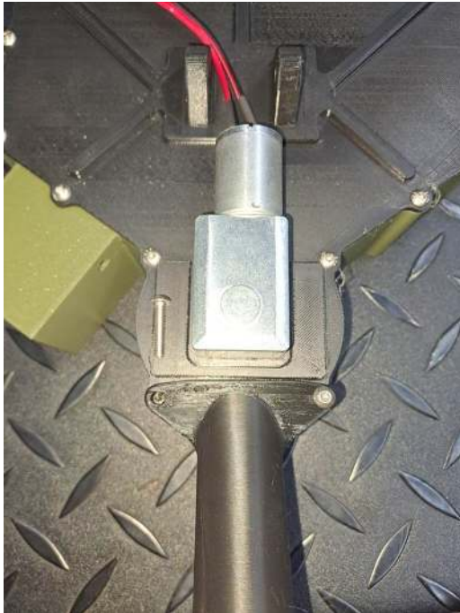
Two long screws used to mount the black funnel.
