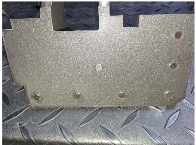
Base magnets fully installed and flush.
