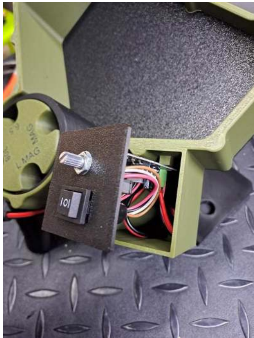
Guide excess wiring into the housing while fitting the panel.
